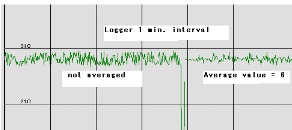
Graph showing the effect of taking average Using T & D product VR71
